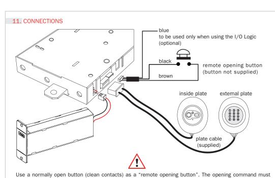
have a duration of less than 1,5 sec. in order to have the pistons and latch always retracted (lock stopped at "daytime opening") provide an opening control with a duration of not less than 20 sec. In order to exit this mode provide the same input with an impulse with a duration of less than 1,5 sec.
