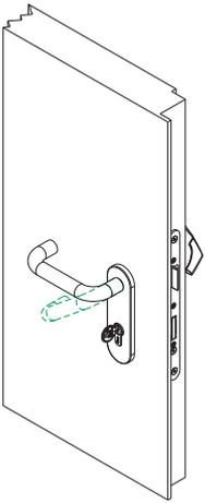
**Catenaccio retracts, door closed only with the latch, external handle enabled.**
